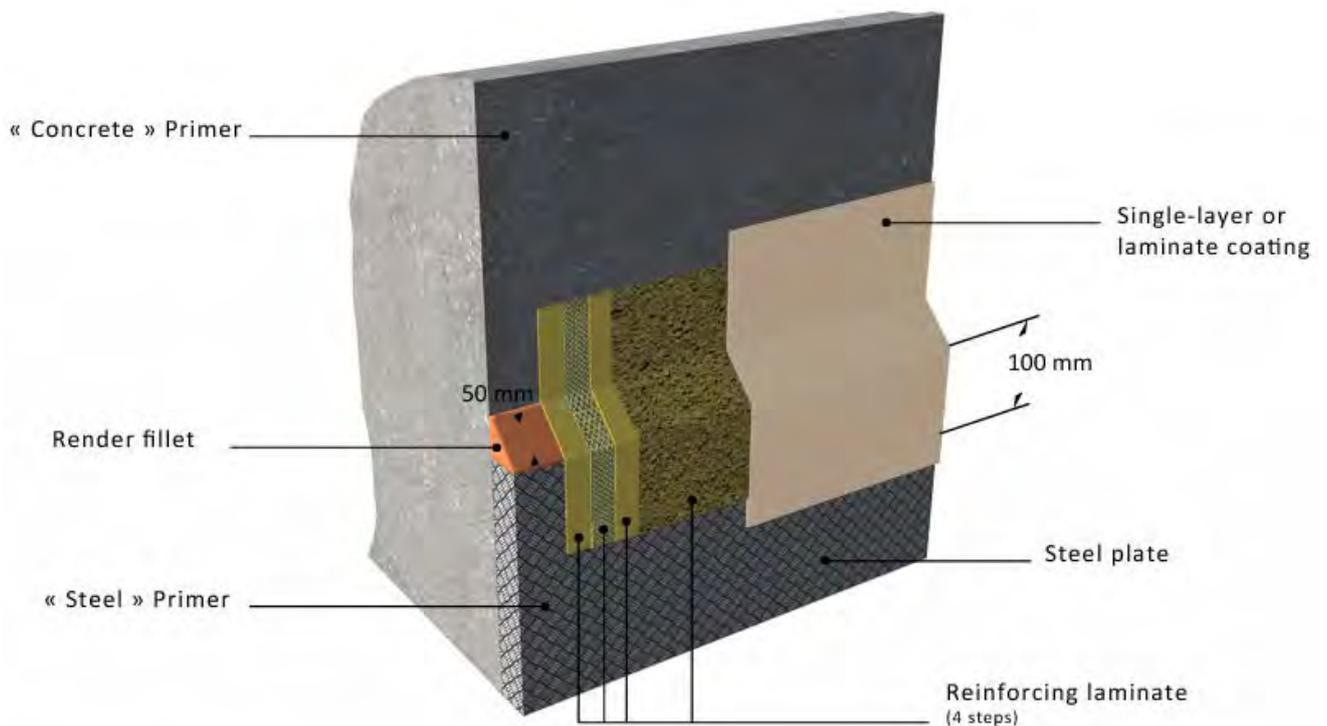
*Sketch no.10: Treating an ingoing steel plate*
