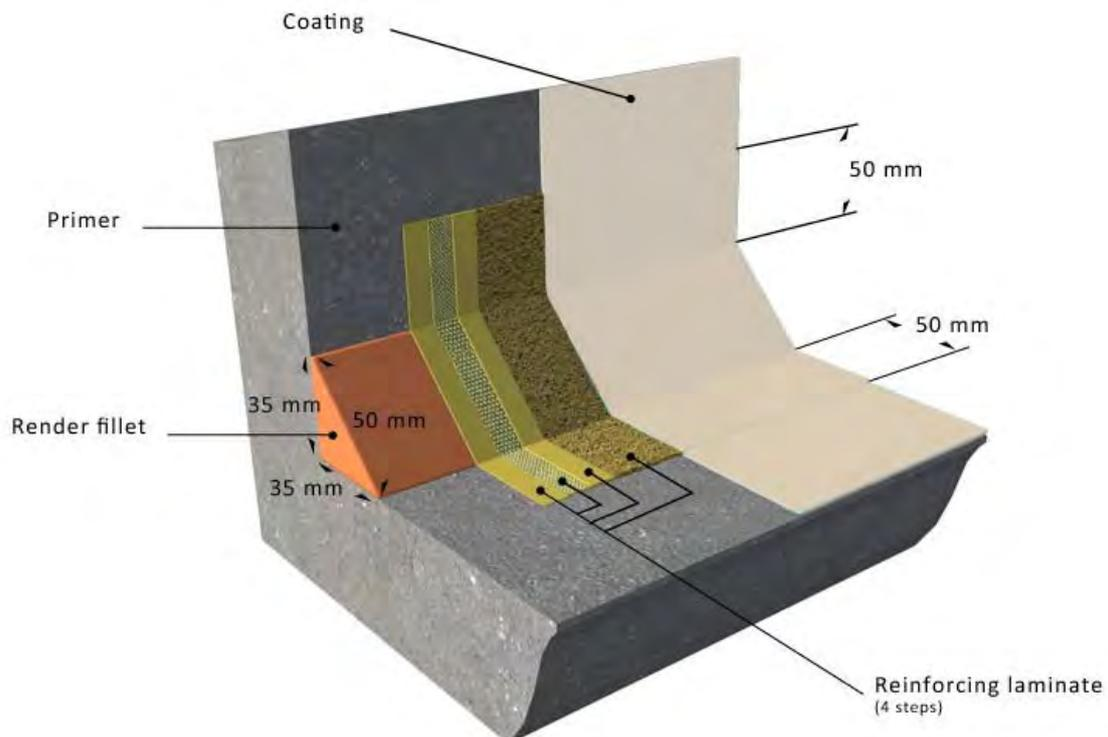
*Sketch no.6: Treating an open angle when applying a laminate coating*
