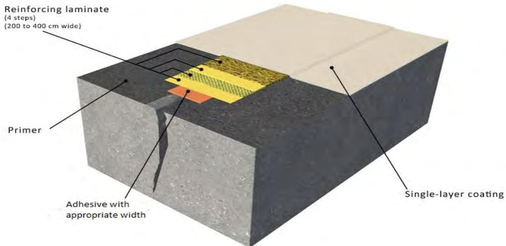
*Sketch no.3: Treating a crack when applying a laminate coating*
