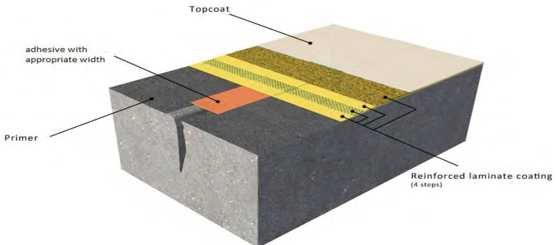
*Sketch no.2: Treating a crack when applying a single-layer coating*
