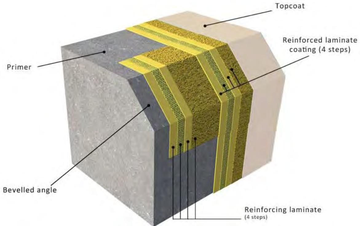
*Sketch no.7: Treating an open angle when applying a single-layer coating*
