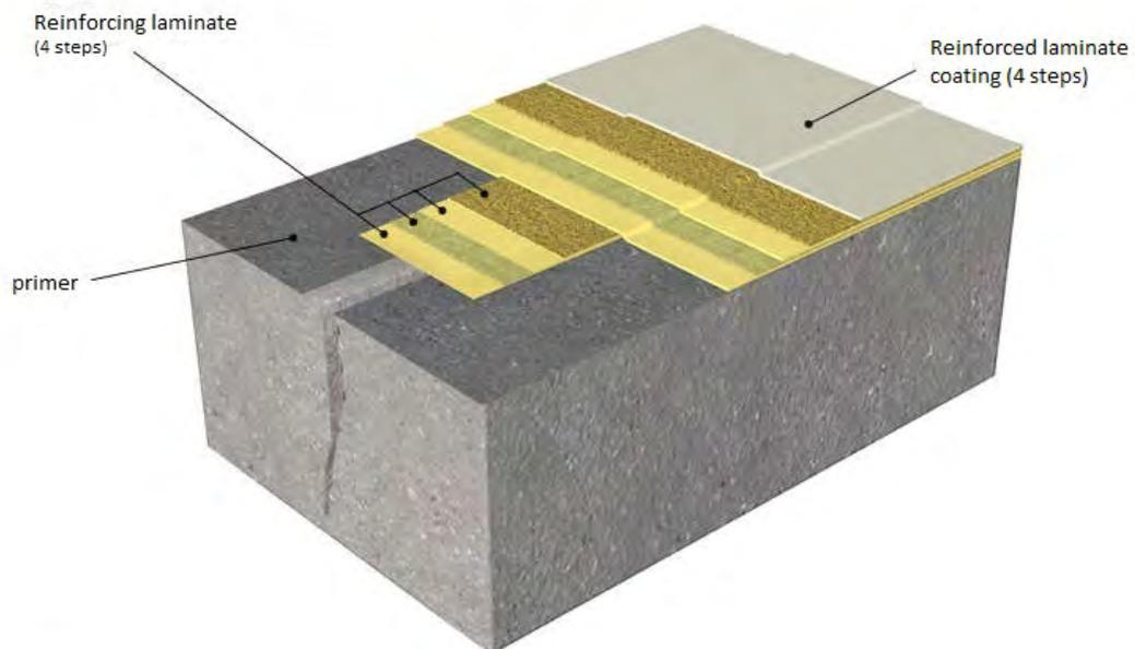
*Sketch no.4: Treating an expansion joint or an active and penetrating crack when applying a laminate coating*
